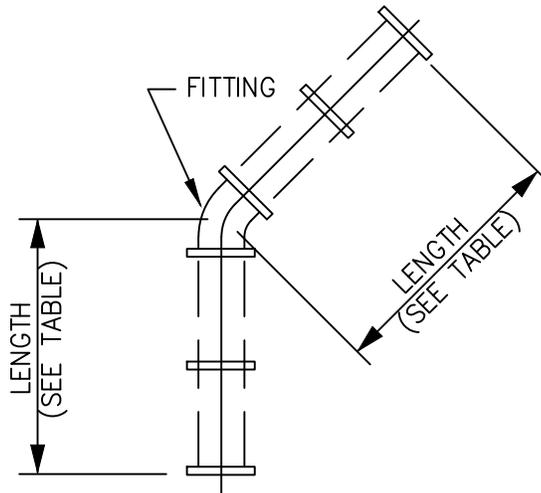
MINIMUM LENGTH (IN FEET) OF RESTRAINED PIPE REQUIRED
