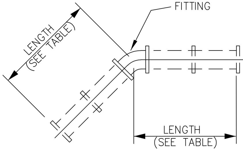
MINIMUM LENGTH (IN FEET) OF RESTRAINED PIPE REQUIRED
